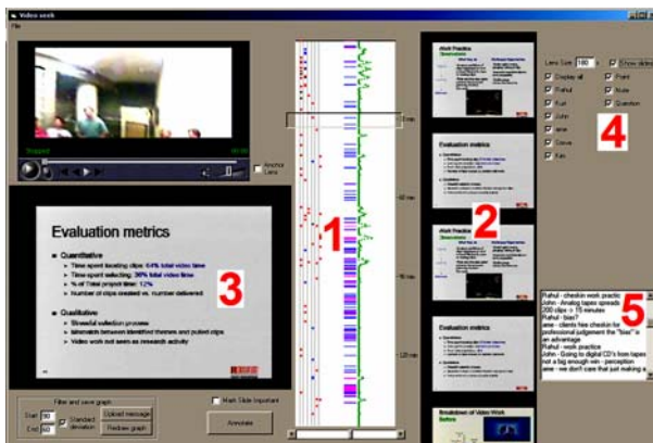
Figure 3. LOI Browser: 1) LOI curve, bookmarks and slide transitions; 2) Thumbnail strip of slides; 3) Slide synchronized to video; 4) Curve filtering options; 5) Full text of user notes
